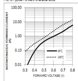
FIG. 2-Typical Forward Characteristics
